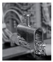
Fig. 4-29: Shield connector terminal with cable
